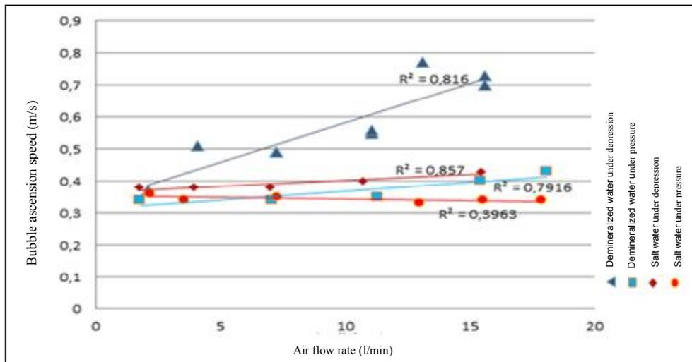
Fig. 7. Bubble velocity for different air flow rates
