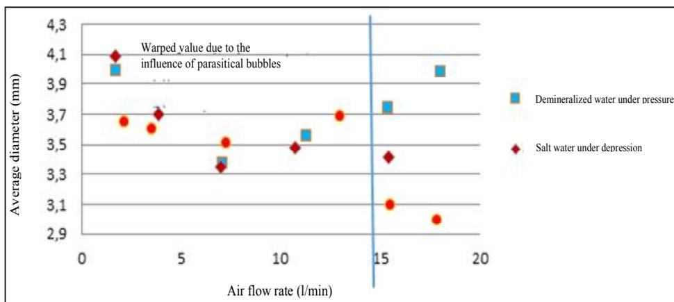
Fig. 5. Bubble diameters for different types of water
