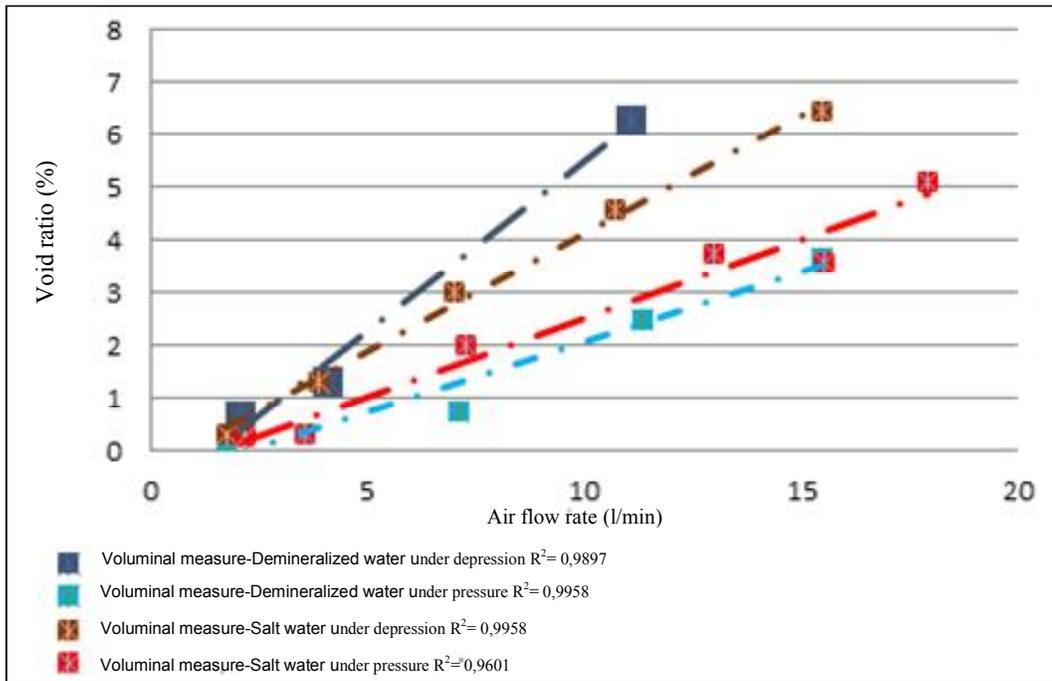
**Fig. 10. Evolution of the empty rate depending on the type of water**
