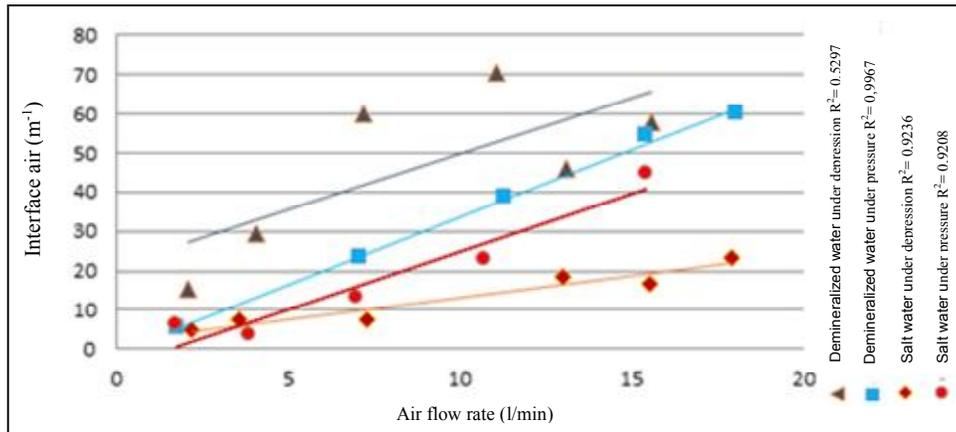
Fig. 8. Variation of interfacial air as a function of air flow
