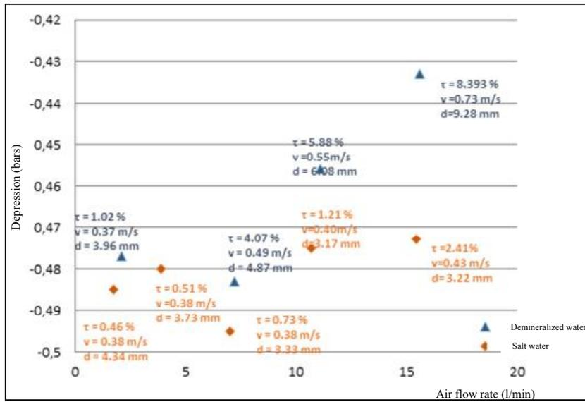
Fig. 3. Pressure variation as a function of flow
