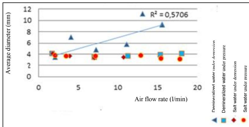
Fig. 4. Average diameters as a function of various water
