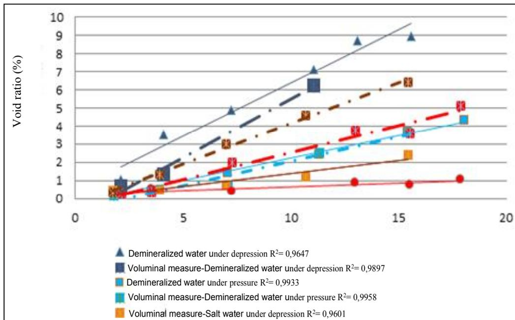
**Fig. 11. Calculation of the vacuum rate as a function of the air flow**
